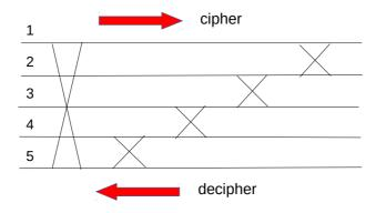
The transposition unit can permute bit 1 and bit 5, bit 4 and bit 5, bit 3 and bit 4, bit 2 and bit 3, bit 1 and bit 2. We represent this by the formule (1-5), (4-5), (3-4), (2-3), (1-2)
